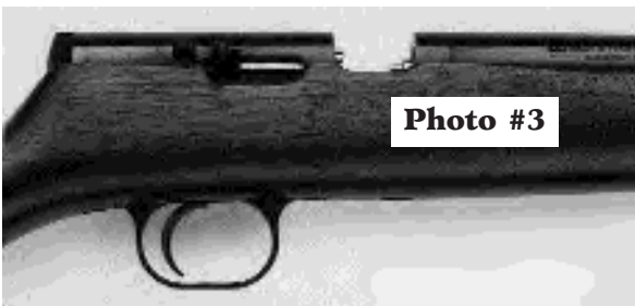
Photo #3 The Striker handle in the "Cocked" Position with the thumb safety in the “Fire” position. The thumb safety will now be in line with the red dot on the stock. A pull rearward on the trigger will now release the striker and cause it to strike the cap on the nipple.
